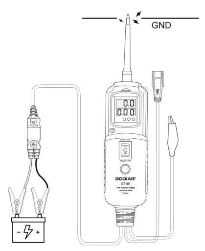
D.Pulse signal communication signal detection: When a pulse signal with voltage is detected, the blue and the red light flash, and the buzzer emits a rapid sound. The voltmeter will display the voltage value of the current circuit.
