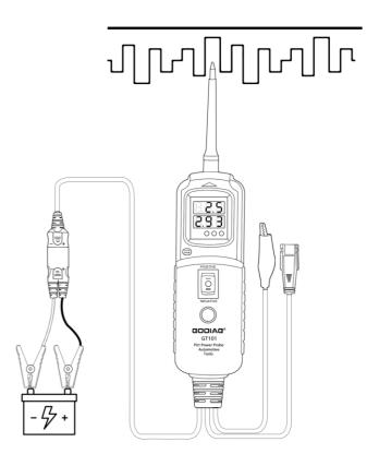
Note: The insulated wire needs to be pierced into and connected to the copper wire by the probe before it can be detected.
